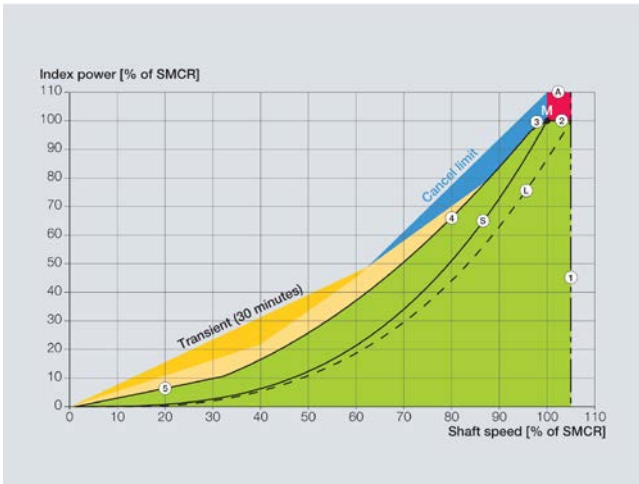
Fig. 7: Traditional and DLF limiters. The area indicated with "Transient (30 minutes)" shows the change in fuel index, shown as power, that becomes available due to DLF. The area indicated with "Increase limit" shows the power that becomes available when using the traditional increase limit button, which is still available and which is working independently of DLF
