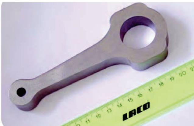
Fig. 4 - Auto connecting rod fabricated via blended elemental approach using hydrogenated titanium powder. Courtesy of Orest Ivasishin, Ukrainian Academy of Sciences
