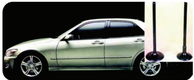
Fig. 5 - The Toyota Altezza (1998 Japanese car of the year) is the first family automobile in the world to feature titanium valves; Ti-6Al-4V intake valve (left) and TiB/Ti-Al-Zr-Sn-Nb-Mo-Si exhaust valve (right). Courtesy of Toyota Central R&O Labs Inc.
