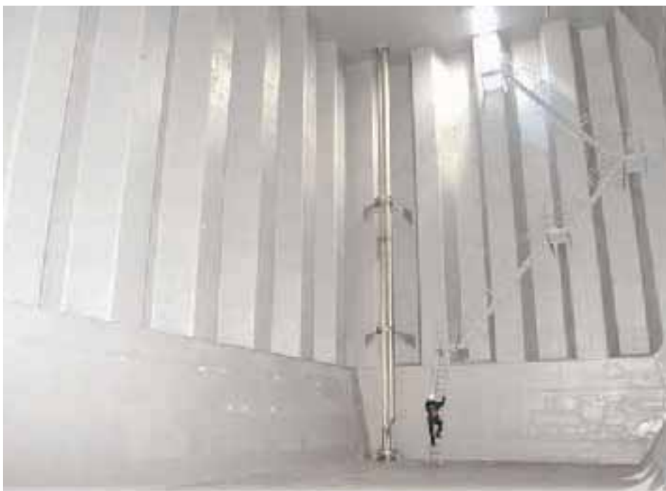
Coated cargo tanks have corrugated bulkheads and no internal structures.
