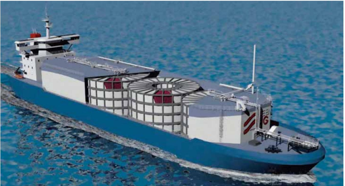
*SeaNG Rendering One of three Compressed Natural Gas (CNG) carrier versions designed by Guido Perla & Associates, Inc. This 118-meter vessel carries 50 mmsCF of CNG in 16 coselles and features a dual-fuel mechanical drive propulsion system.*
