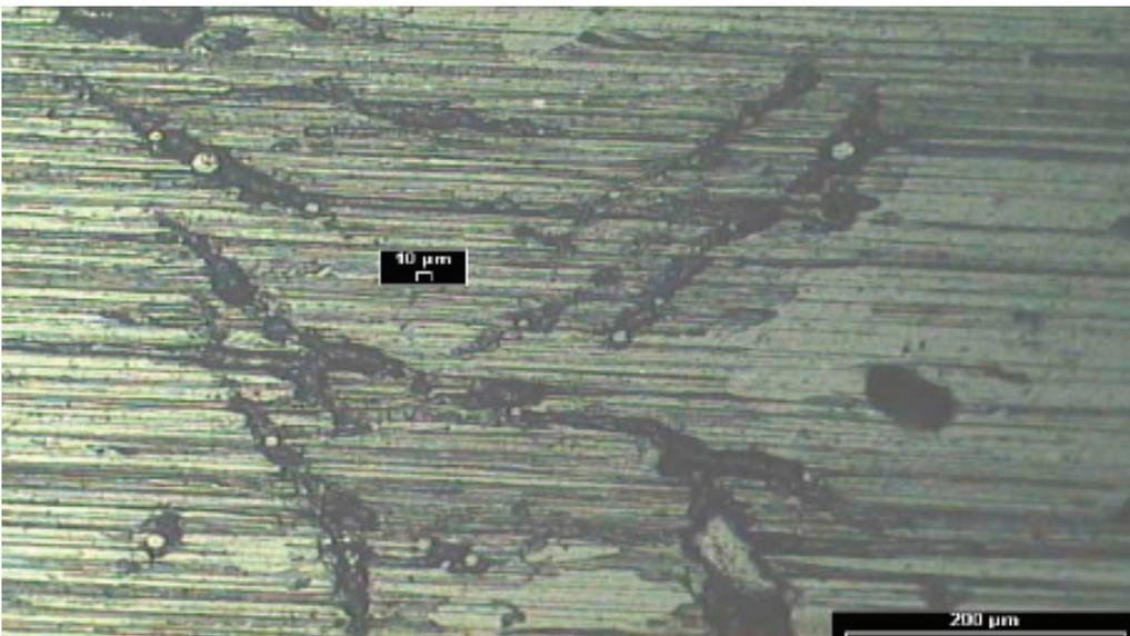
*Figure 3. Wear on a cylinder liner.*
