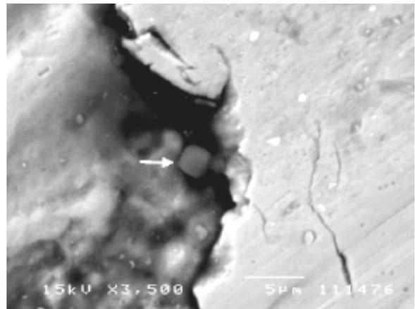
*Figure 1. Fuel pump spindle guide with scuffing and excessive wear.*
