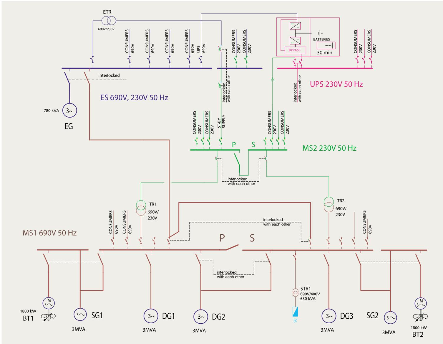
Fig. 2 – Low-voltage 690V network for auxiliary power station: diesel-mechanical propulsion.
