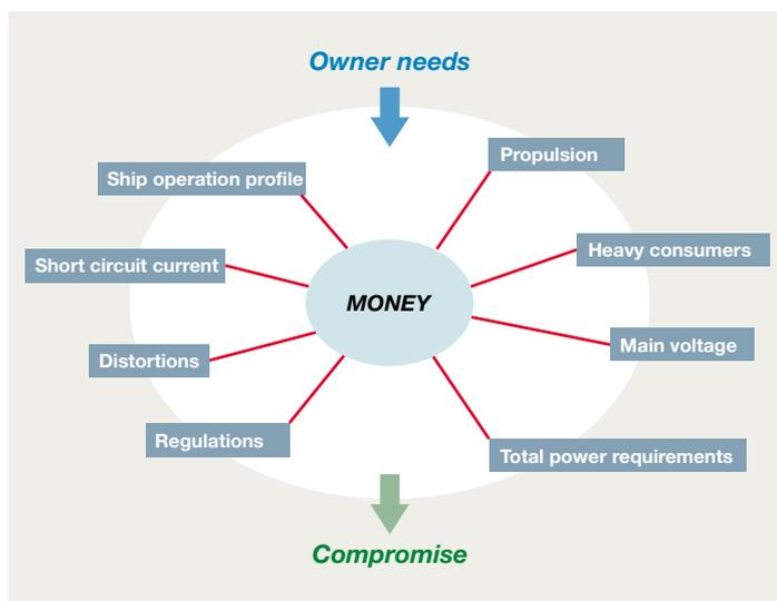
Fig. 1 – Designing a ship's electrical network calls for a careful balance of various critical factors.
