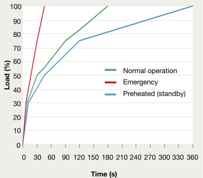
Fig. 5 – Typical engine (Wärtsilä 46) maximum loading
