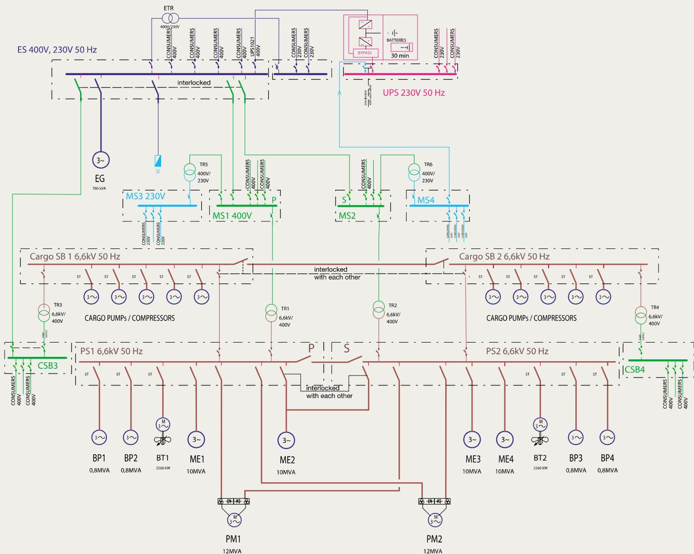
Fig. 3 – Medium-voltage 6.6kV network for a main power station: electric propulsion of an LNG tanker.
