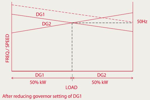
Fig. 4 – Load sharing in speed droop mode.
