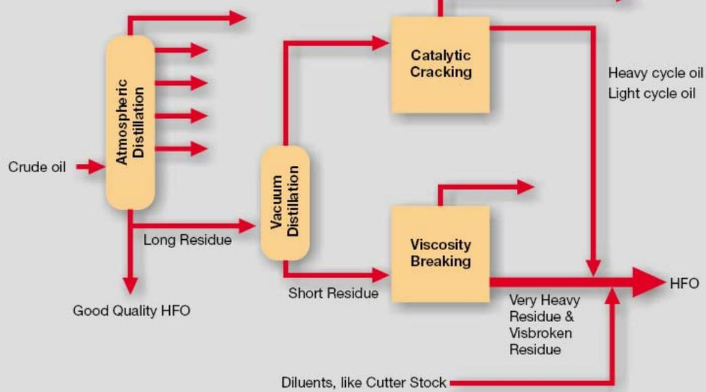
Fig. 2 Example of modern fuel refinery configuration.
